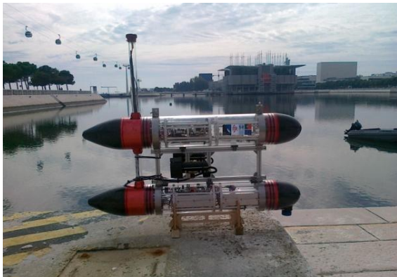
The MEDUSA semi-submersible autonomous marine robot at the EXPO 98 testing site (first prototype)
