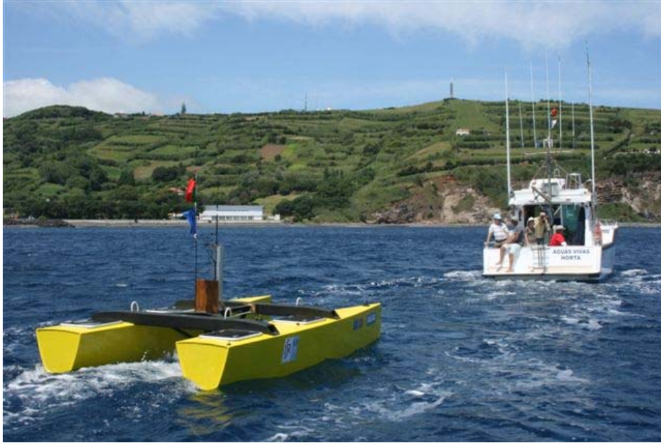
The DELFI-Mx Autonomous Robotic Vehicle Following the “unknown” AGUAS VIVAS target: first experiments of cooperative motion control in the Azores, in the scope of the European GREX project.
