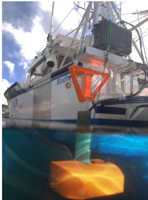
Multibeam Sonar (IST/ISR) installed in the AGUAS VIVAS vessel, property of IMAR/DOP/UAçores.
