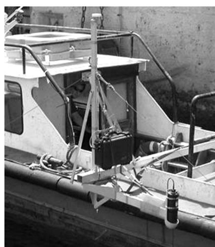
Figure 3. The IRIS high accuracy measuring device. a) Detail of the mechanically scanned high aperture sonar profiler; b) View of IRIS installed in the support vessel.
