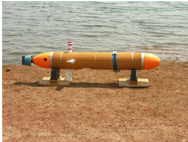
The MAYA AUV - Mechanical Design of the NIO, India
