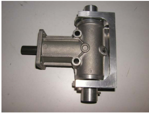
a) Gearing system for a revolution joint
