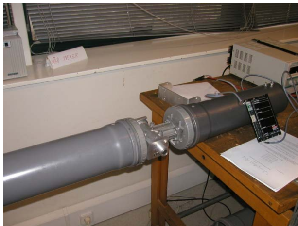
Figure 8: Setup for testing the flexibility of a 2-link arm
