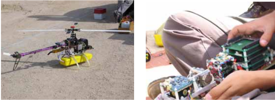
Figure 1. Vario Xtreme Helicopter equipped with control electronics. Left) Helicopter ready to takeoff; Right) Detail of the control electronics and motion sensors.
