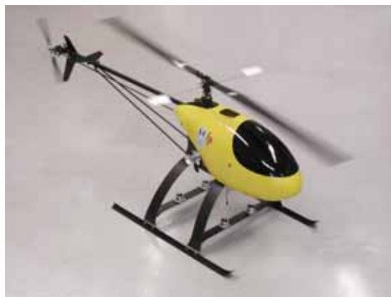
Figure 2 Bergen Industrial Twin Helicopter with modified landing gear.
