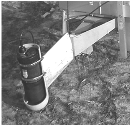
Figure 3. The IRIS high accuracy measuring device. a) Detail of the mechanically scanned high aperture sonar profiler; b) View of IRIS installed in the support vessel.
