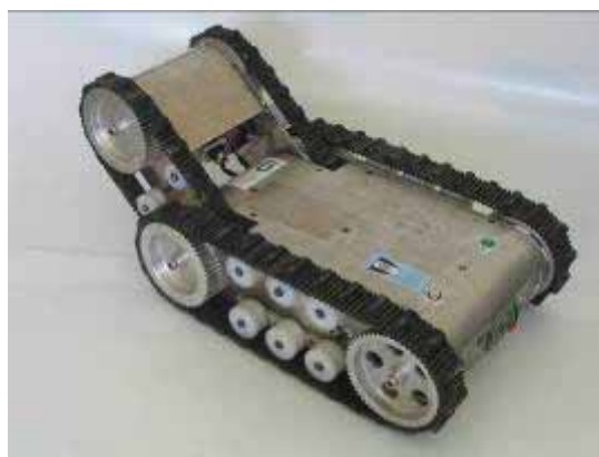
RAPOSA Rescue robot, developed together with Portuguese companies IdMind and SetPontes, within the framework of the AdI Project RAPOSA
