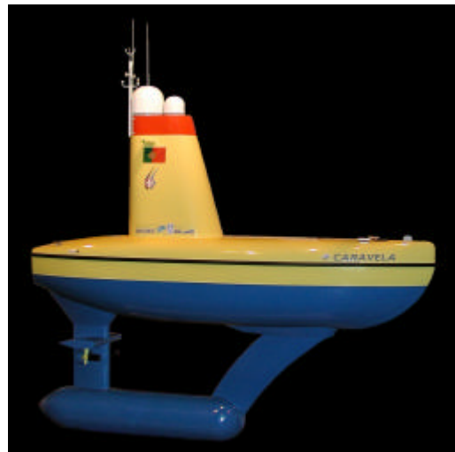
The CARAVELA Autonomous Surface Craft (ASC): CAD figure and scaled down model (to be launched in April 2003)
